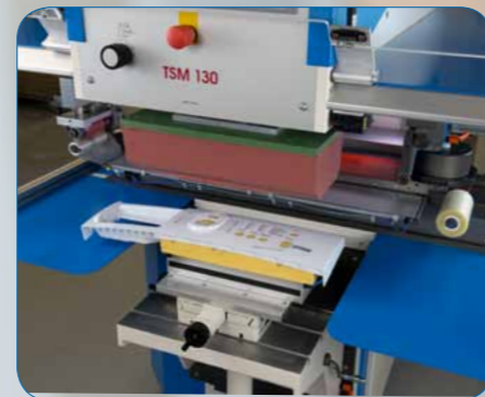
TSM 130 universal transverse doctor kit with “ink residue pick-up system”
