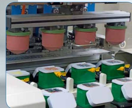
TSM 60/90 universal multiple colour kit Solo 4-colour printing
