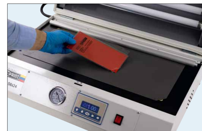
Cliché, film assembly plate and film are placed inside the exposure unit
