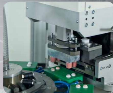
Automation with 4-fold use 36.000 parts/h
