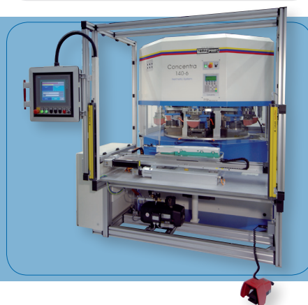
Semi-automatic machine for washing machine panels
