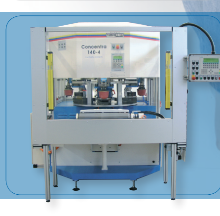
Semi-automatic machine for "white goods" (w-x-y-z + r axes)
