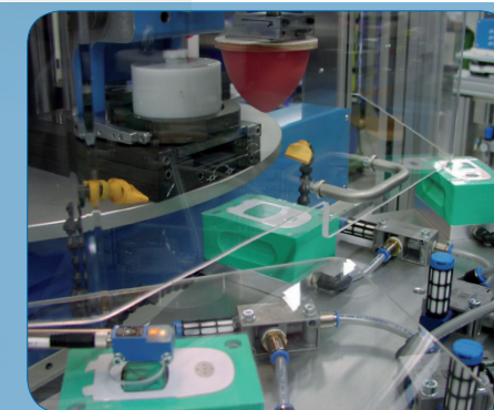
CONCENTRA 90-4 with rotary index table, jig with vacuum support
