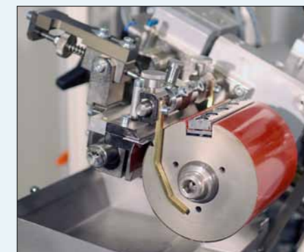
Fig.: Clamping cylinder mounted in rotary pad printing unit
