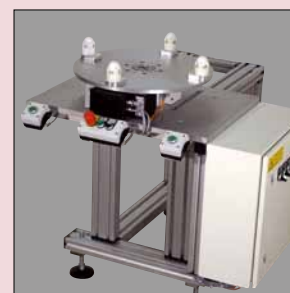
^ Aluminium profile with rotary index table T4
