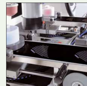
Integrated laser unit for production of printing clichés
