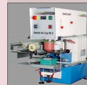
^ With fitted ink residue pick-up system
