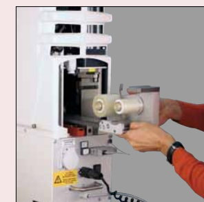
^ Ink residue pick-up system (pad cleaning)
