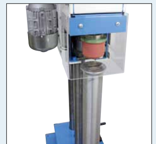
Example for utilization of the large working area: Printing on the face of a cylinder
