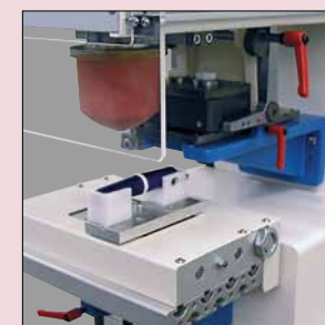
^ With fitted single jig carrier (hand-work place)
