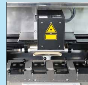
^ Linear motor axis with receiver plate for 4-colour screen set
