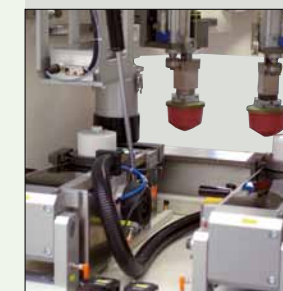
2 printing stations equipped with microflex cliché band
