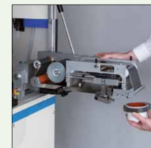
Slewable printing unit for the easy exchange of cliché band and ink
