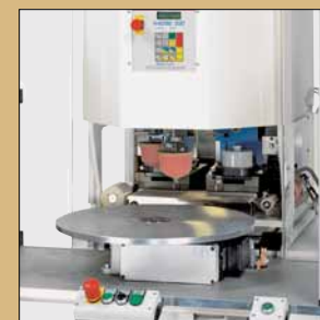
^ T2 rotary index table for the feeding of workpieces
