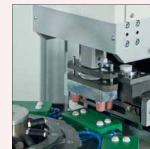
^ Fully automated system with 4-way use = 36,000 parts/h
