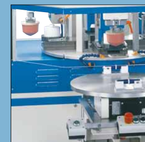
^ Rotary index table T2 for the parallel feeding of work-pieces
